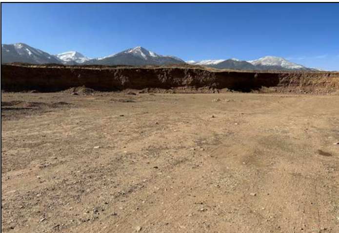
Photos 3 and 4 - Working face high wall on west end of affected area is larger than the currently approved 400' long by 10' high.
