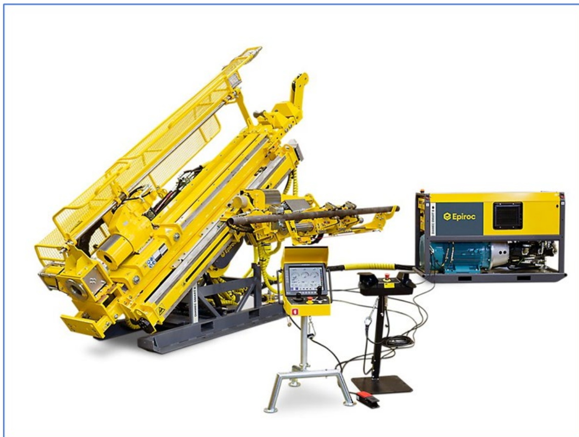
Figure 3. Diamec U-8 Core Rig showing Electrical Controls
