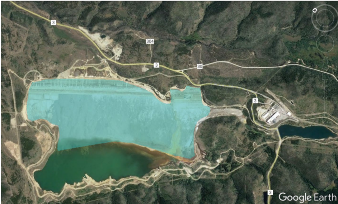
Figure 2. The Henderson Tailings Storage Facility consists of dry tailings impoundment (shaded light green) and reclaim pond (dark green). The dry beach and embankment are treated with Coherex to suppress dust mobilization.
