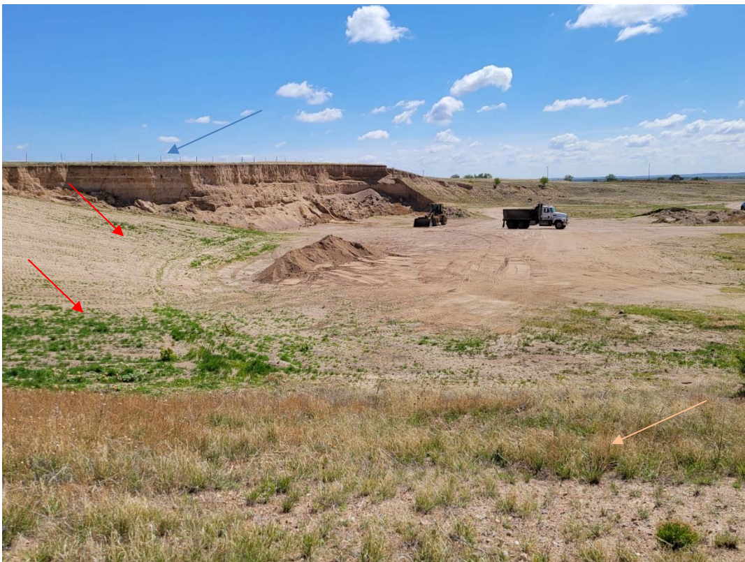
Looking east across excavated pit. Red arrows point to recently graded and seeded area. Small stockpile of mined material in pit. Fence line at top of highwall is the northern permit boundary. Older reclaimed area in foreground.
