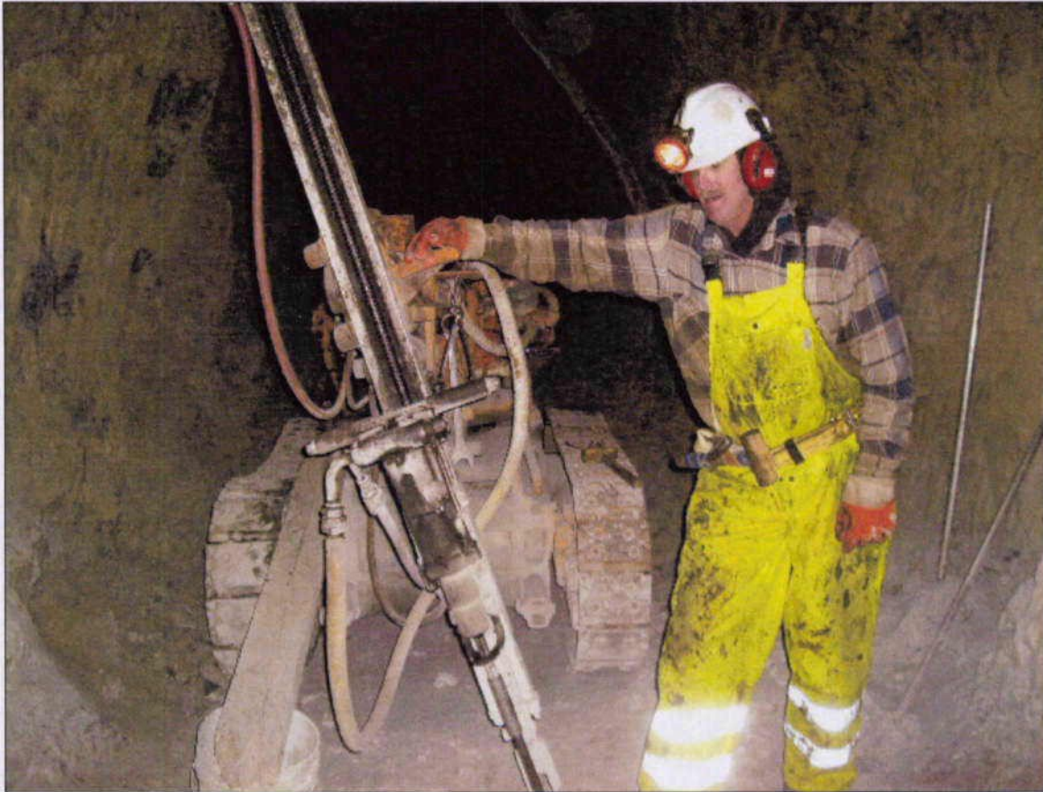
Figure 3: Probe hole drilling in Pierce adit floor
