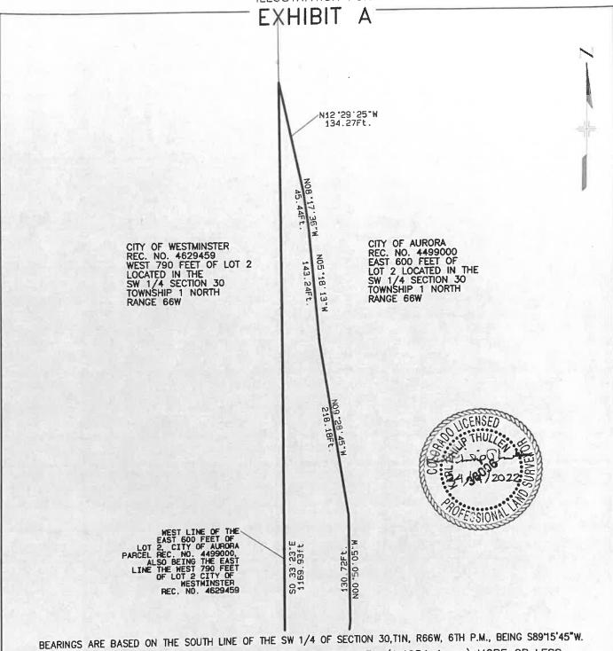
BEARINGS ARE BASED ON THE SOUTH LINE OF THE SW 1/4 OF SECTION 30,71N, R66W, 6TH P.M., BEING S89"15"45"W.
