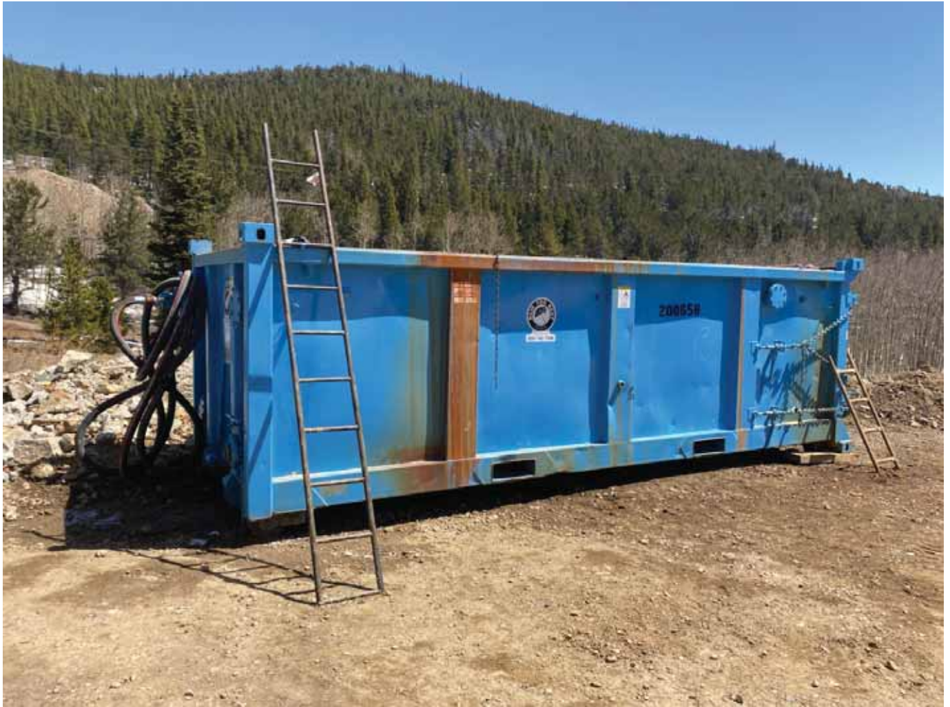
Figure 16 Current Backwash and Settling Tank
