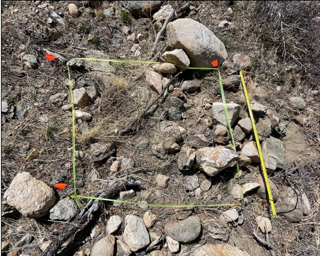
Figure 3. Southwest facing CCP fill slope approximately 170 feet below the Parkway. Tape measuring = 5' in length; total 25 square feet area. View looking east up the slope.
