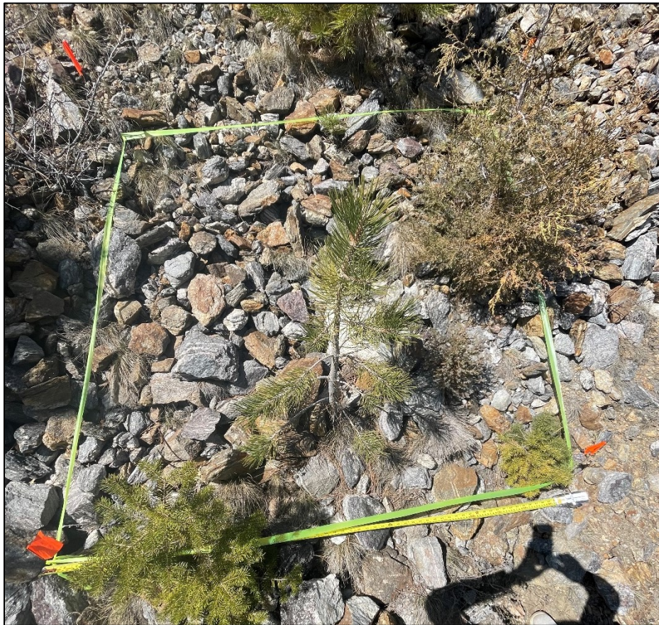
Figure 1. East-northeast facing CCP fill slope approximately 170 feet below the Parkway. Tape measuring = 5' in length; total 25 square feet area. View looking west up towards the CCP.
