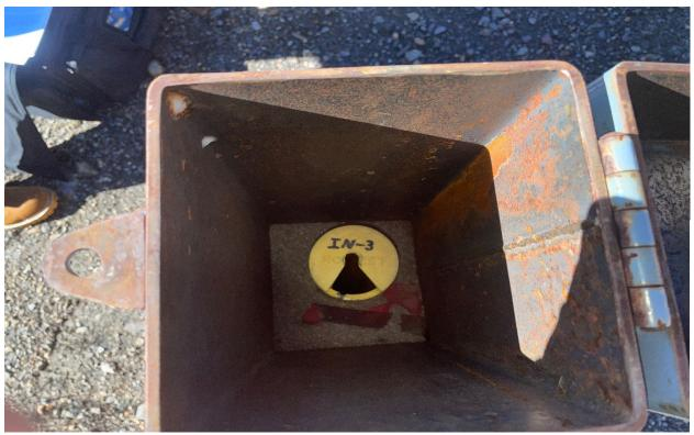
Photo 1: Handmade cable catch used when pulley could not be used
