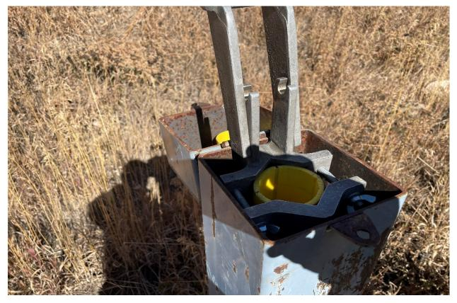
Photo 4: Pulley mechanism used for accessible casings
