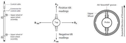
Figure 2-1: Inclinometer Probe and Casing directions
