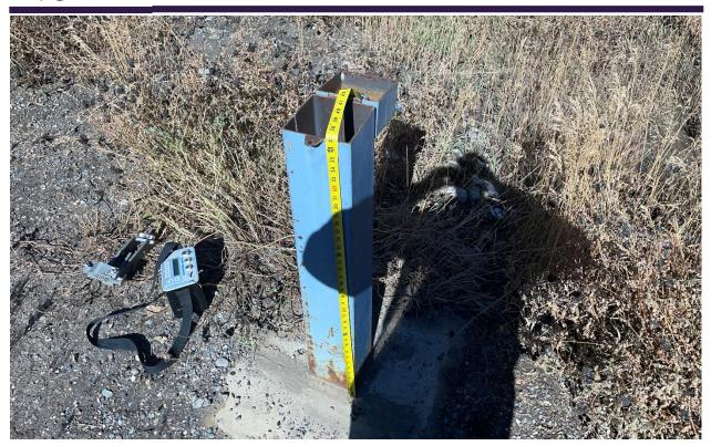
Photo 3: Stickup of casing, measured from concrete base
