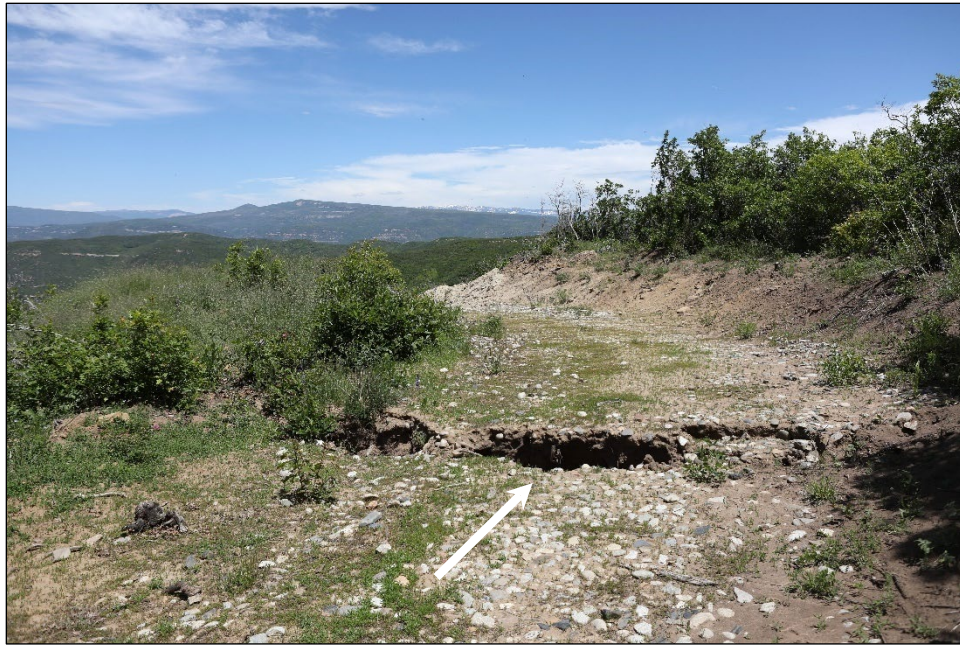
Figure 3. Northward view during the spring 2019 field visit of a subsidence crack (see white arrow) with 6-inch elevation change from north to south observed approximately 1,000 feet north of the MVB E6-14 pad.
