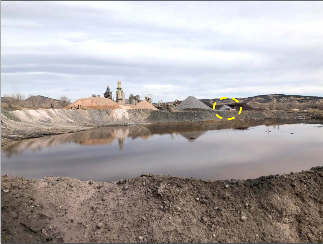
Photo 3. View looking north across northeastern unbackfilled portion of Pit C with ponded water. Note water truck (circled in background) spraying raw material stockpile area located north of Pit C.
