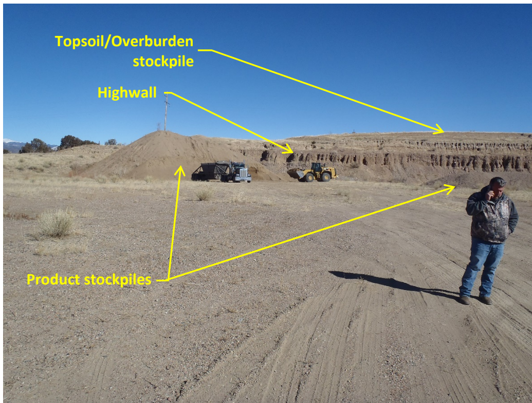
Photo 2. West end of highwall, product stockpile & overburden/topsoil (looking NE).
