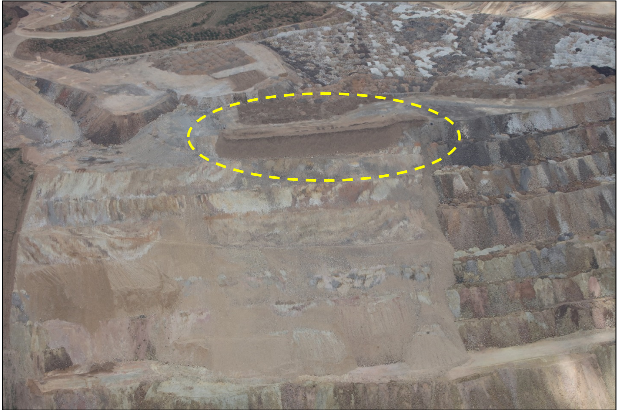
Photo 8. 2021 concurrent reclamation area on the ECOSA, staged topsoil circled; looking southwest.
