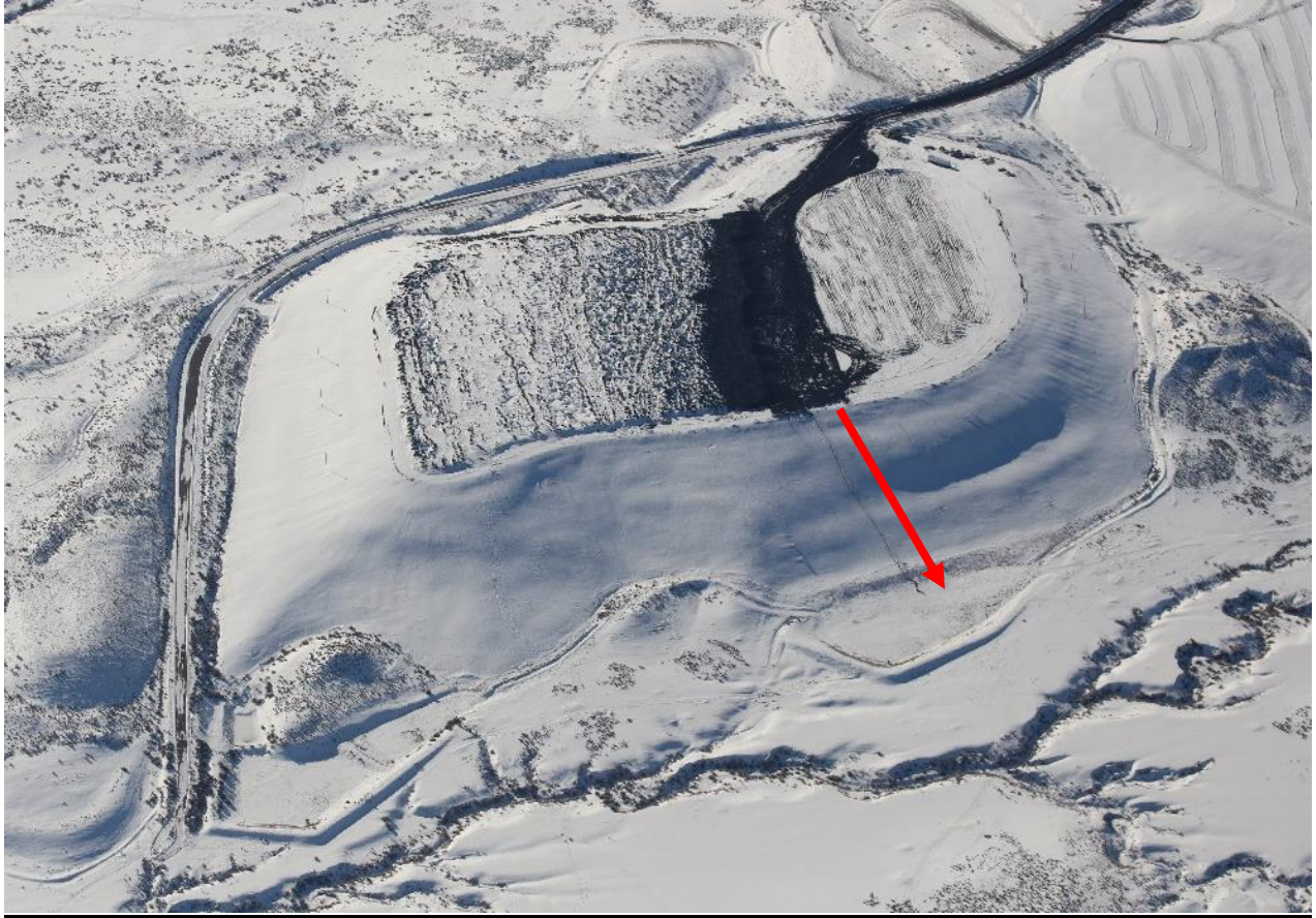
Photo 3: The RP-2/3/4 refuse pile. The large rill is shown next to the red arrow in the photo above.
