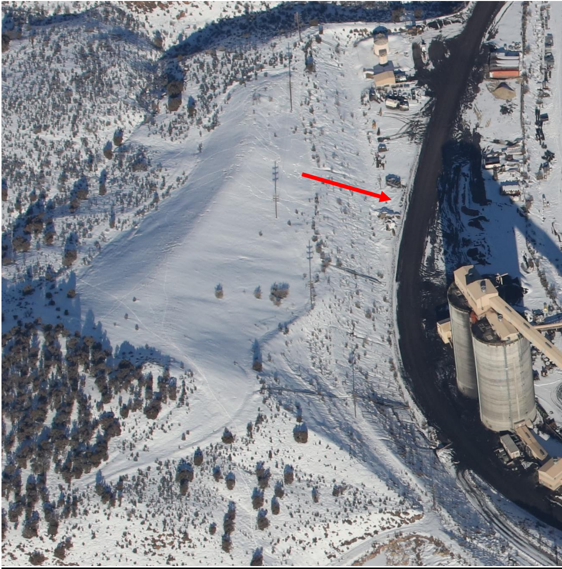
Photo 4: The large rill located on the slope below the main facilities/portals area topsoil pile. The rill is just below the perimeter ditch, shown above the red arrow in the photo above.
