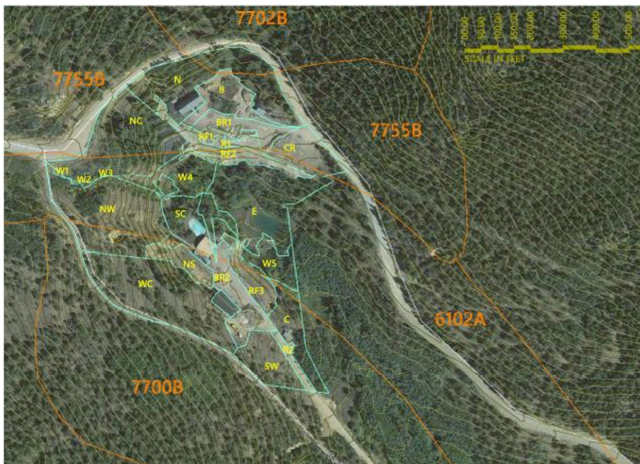
Figure 2 Outlines of sediment generation areas from the Stormwater Management Plan.
