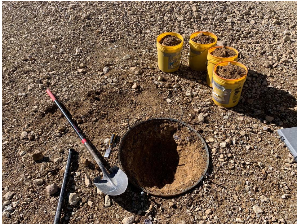
November 11, 2021 – High Compaction Backfill water volume replacement excavation (TW)
