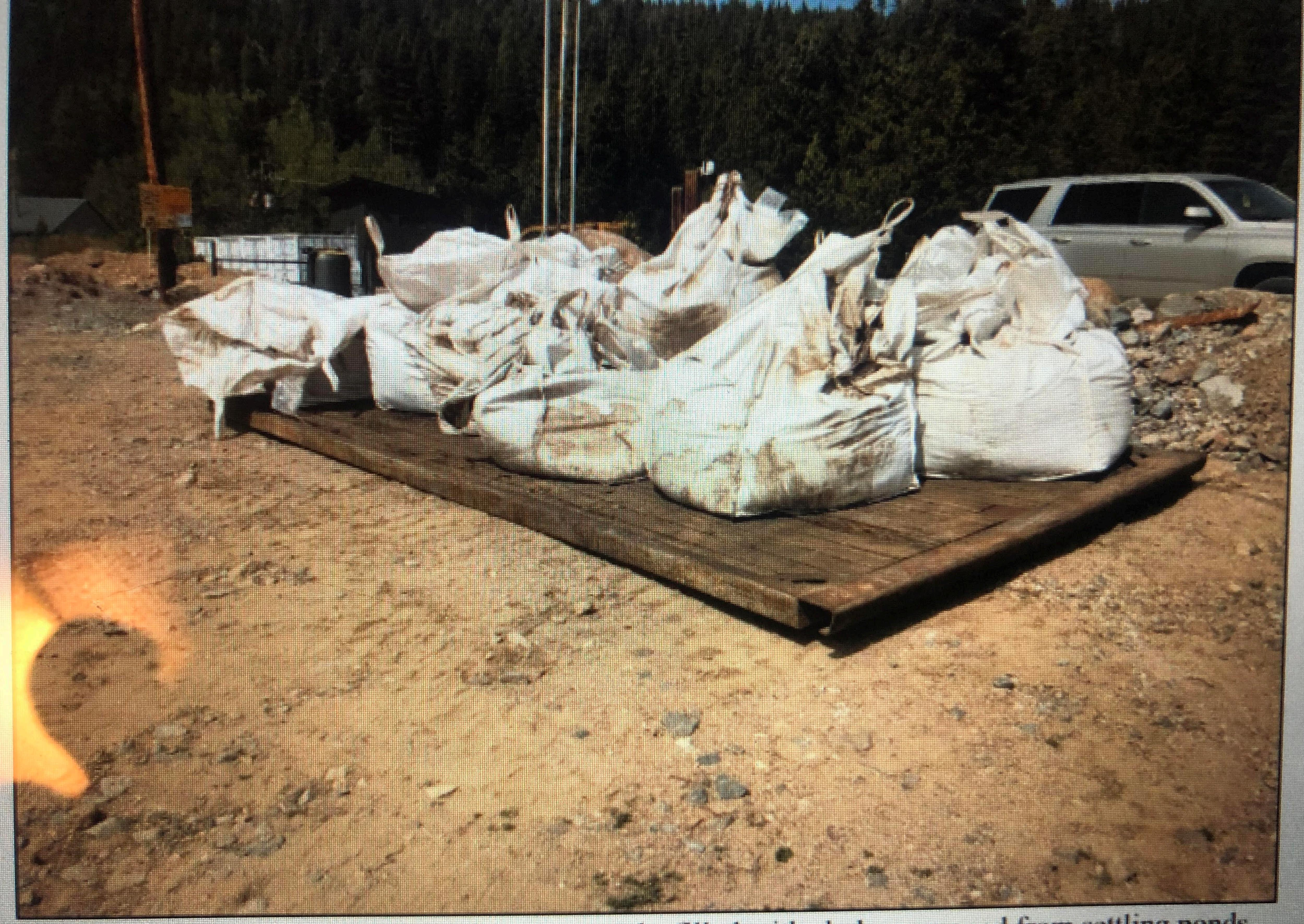
Photo 47. View looking north at nine super sacks filled with sludge removed from settling ponds, currently stored on top of existing waste rock pile in Caribou Mine area. Operator will need to perform additional lab testing on this material to determine an appropriate disposal location.
