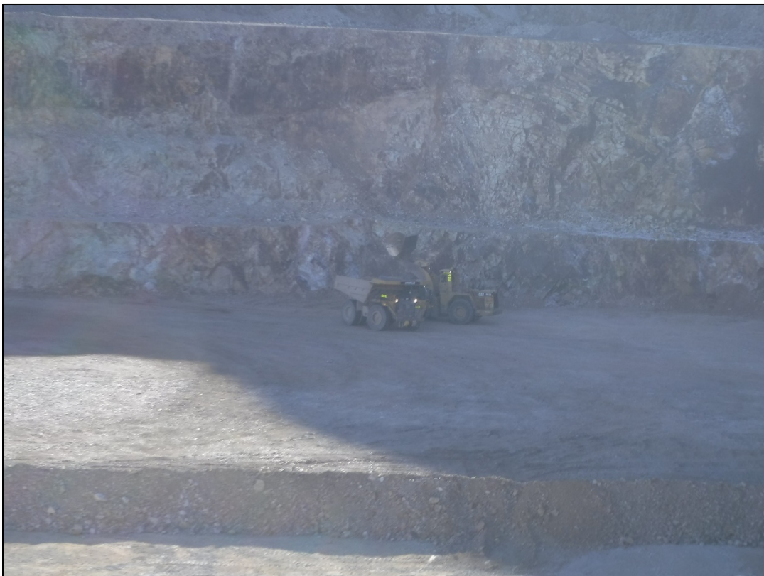
Photo 6: Removal of oversized material from lift
