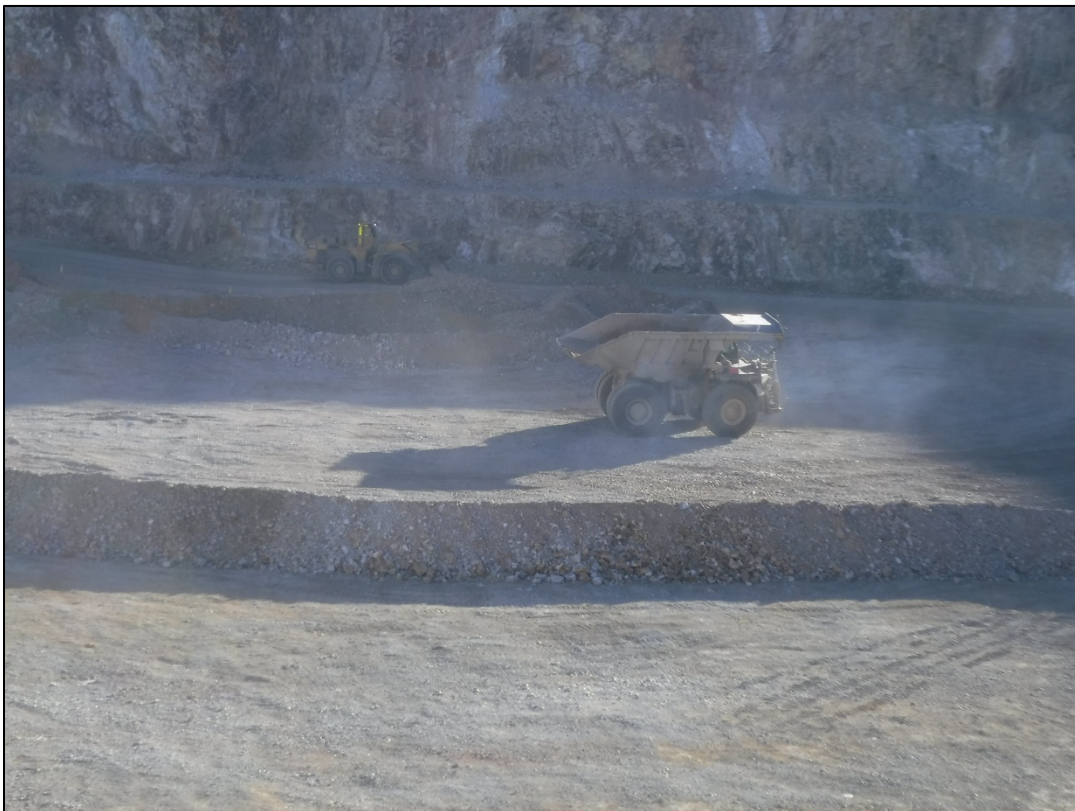
Photo 4: Haul truck leaving dump area, note even spread of tire tracks across lift area
