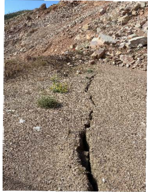
2. CRACKING NEAR PRODUCTION FLOOR
