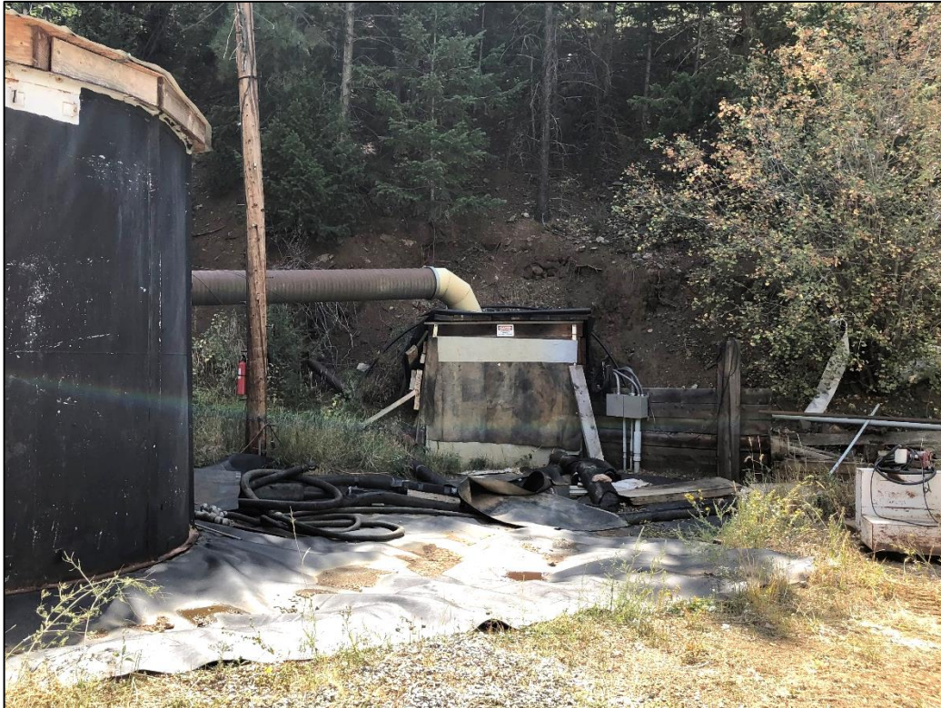
Photo 3. View looking west/southwest at Steve Adit, located just northwest of water treatment plant on top of mesa. Mine water was previously pumped from this adit to treatment plant. However, mine water is now pumped from Jeffrey Air Shaft located on hillside above treatment plant. It is not clear what continued use the operation has for this adit and what infrastructure remains inside.
