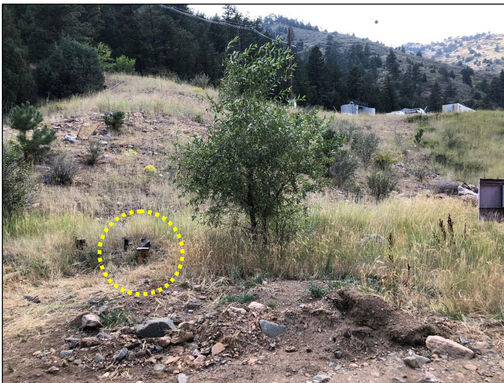
Photo 8. View looking west/northwest at alluvial groundwater monitoring well MW-6 (located southeast of mesa with water treatment plant), which operator may propose (in an upcoming Technical Revision) to abandon, if alluvial material surrounding well must be removed for valley excavation project.
