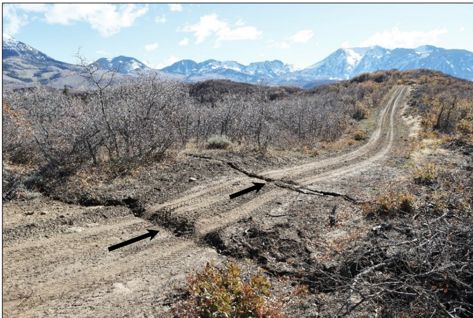
Figure 1. Southeastward view during the fall 2018 field visit of two parallel subsidence cracks that appeared as a result of recent longwall mining beneath the area. The closer crack showed more rounded edges than the distant crack, suggesting the latter was more recently formed.
