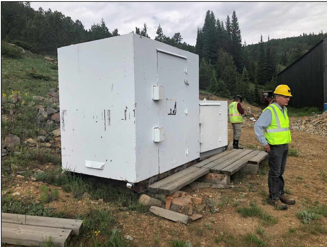
Photo 8. View looking northwest at explosives storage area located southeast of Cross Warehouse/Ore Storage Building in Cross Mine area, where two magazines are secured with padlocks and lock boxes.
