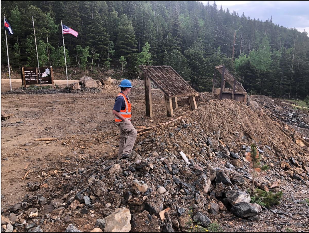
Photo 37. View looking northeast across top of historic waste rock pile located in Caribou Mine area. Rock screens were present in this area during inspection. Operator is not authorized to conduct any processing activities on site beyond screening/sizing waste rock for aggregate use.
