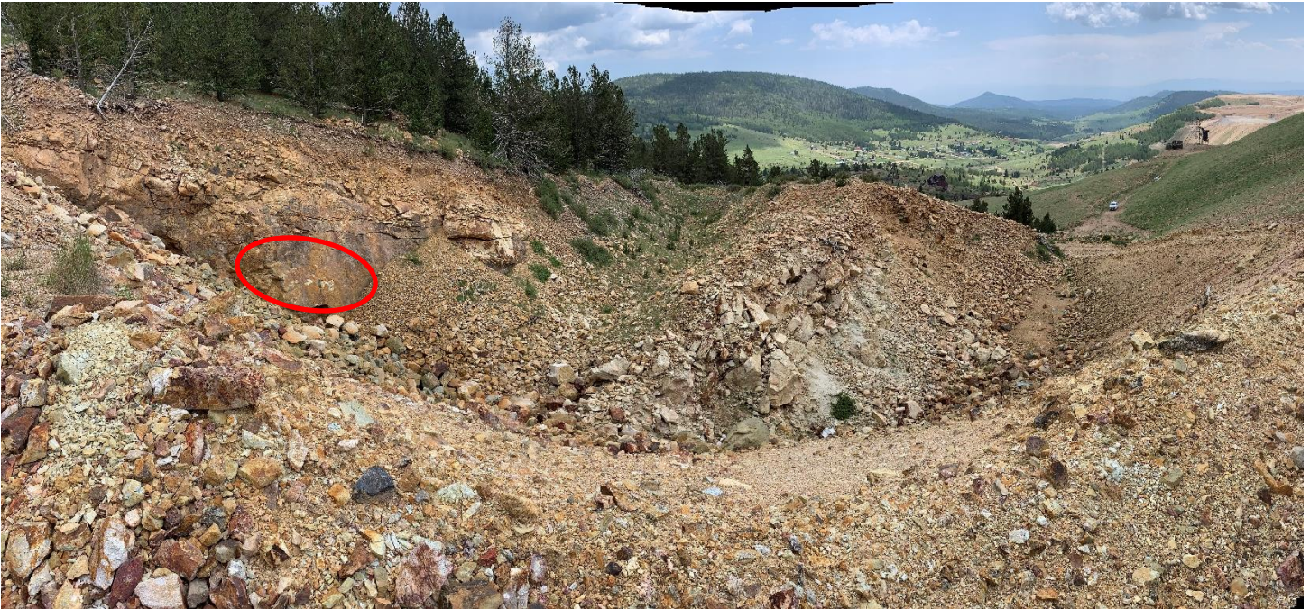
Photo 14 – Altman Backfill hole facing south, with blast holes
