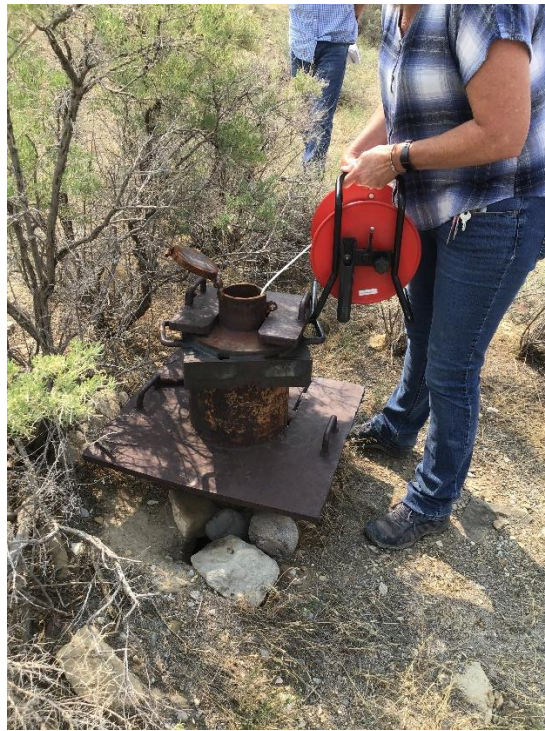
Photo 5: Tonya Hammond using a Solinst Model 101 water level meter at the N1 Well.
