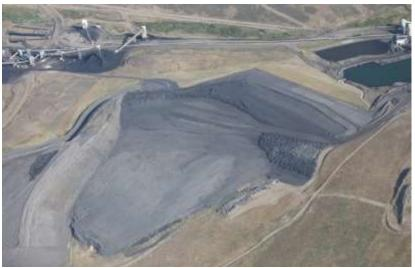
Photo above shows the waste pile, pond D and the pit pond at the top right, pond B at the top left. Ponds B and D appear to need to be cleaned. No issues are noted with the waste pile.
