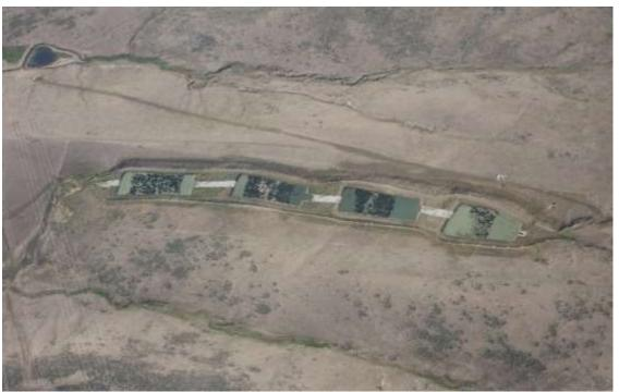
The passive treatment ponds near the 6MN reservoir are shown above. Wetland plants appear to be establishing well. Flow in the photo is from right to left. The system does not appear to be discharging at the time of the photo. Vegetation on the banks around the system appear to be improving. No cattle appear to be present within the fenced area. Slopes and rock check dams in the diversion ditches appear stable.
