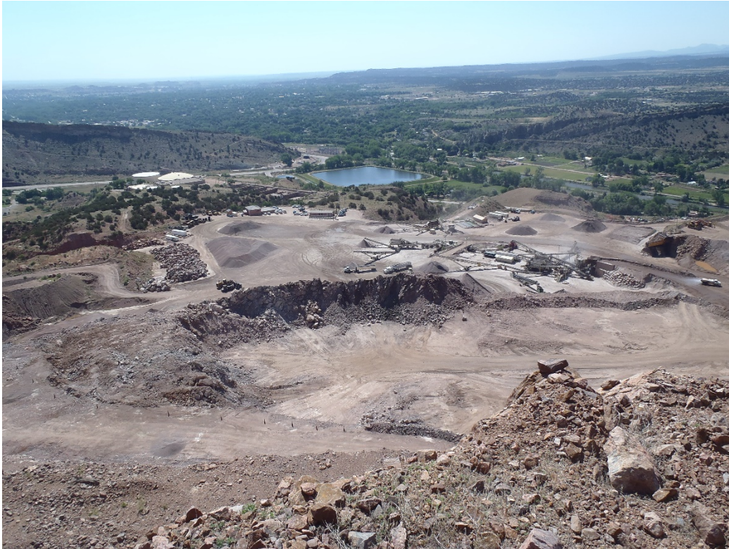
Photo 4. Pit floor from the phase 2 north highwall (note screen plant, loader, haul trucks - looking south).
