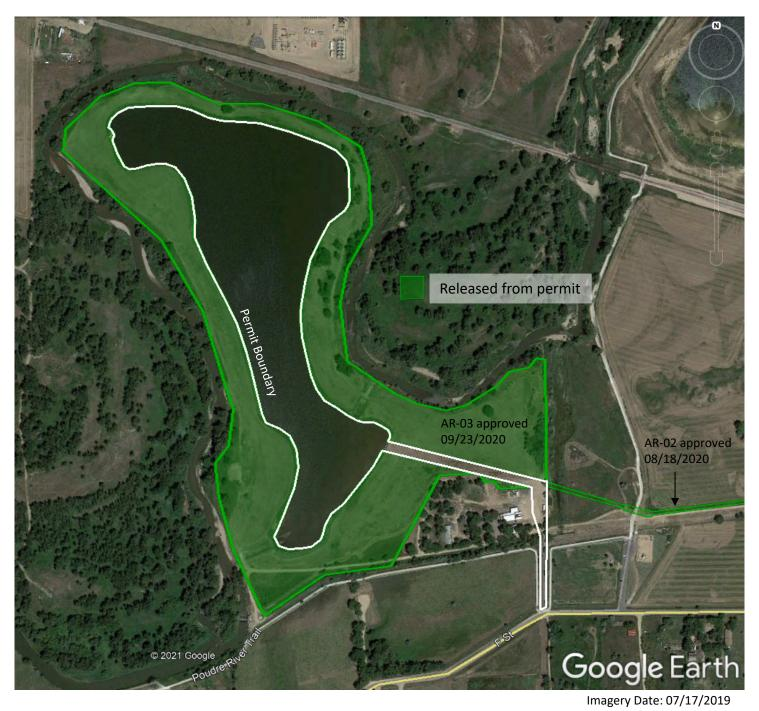
All disturbed areas have been graded, topsoiled and seeded above the water table.
