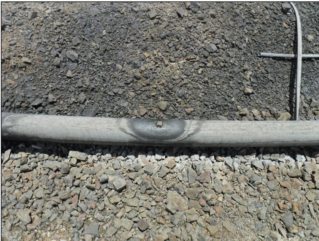
Photo 24: Typical plug that failed, all plugs are gradually being cut out and replaced by fusion welds
