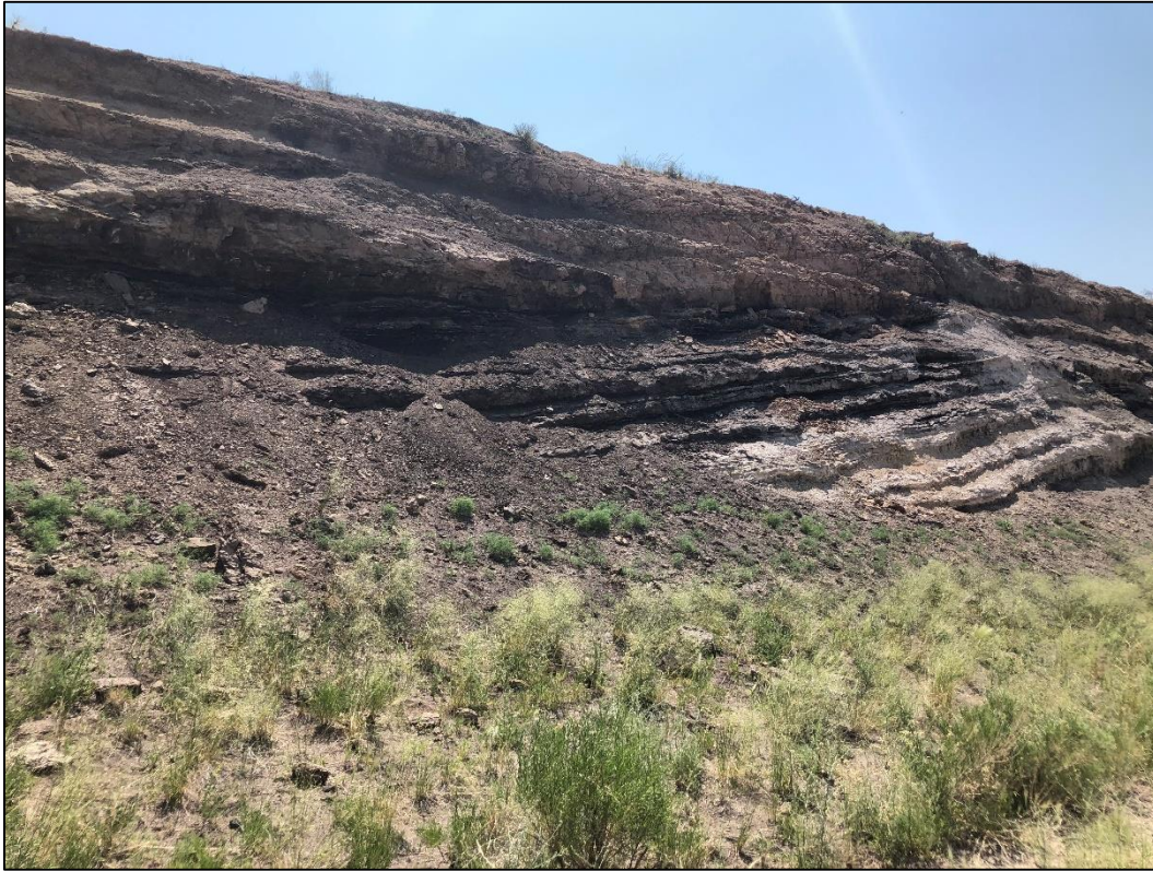
Photo 17. Closer view of eastern highwall of East pit, approximately 15-20 feet in height with near vertical to 1H:1V slopes.
