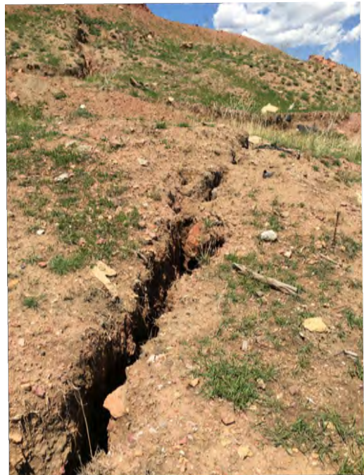
7. HEALED CRACKING PARRALEL TO SLIDE
