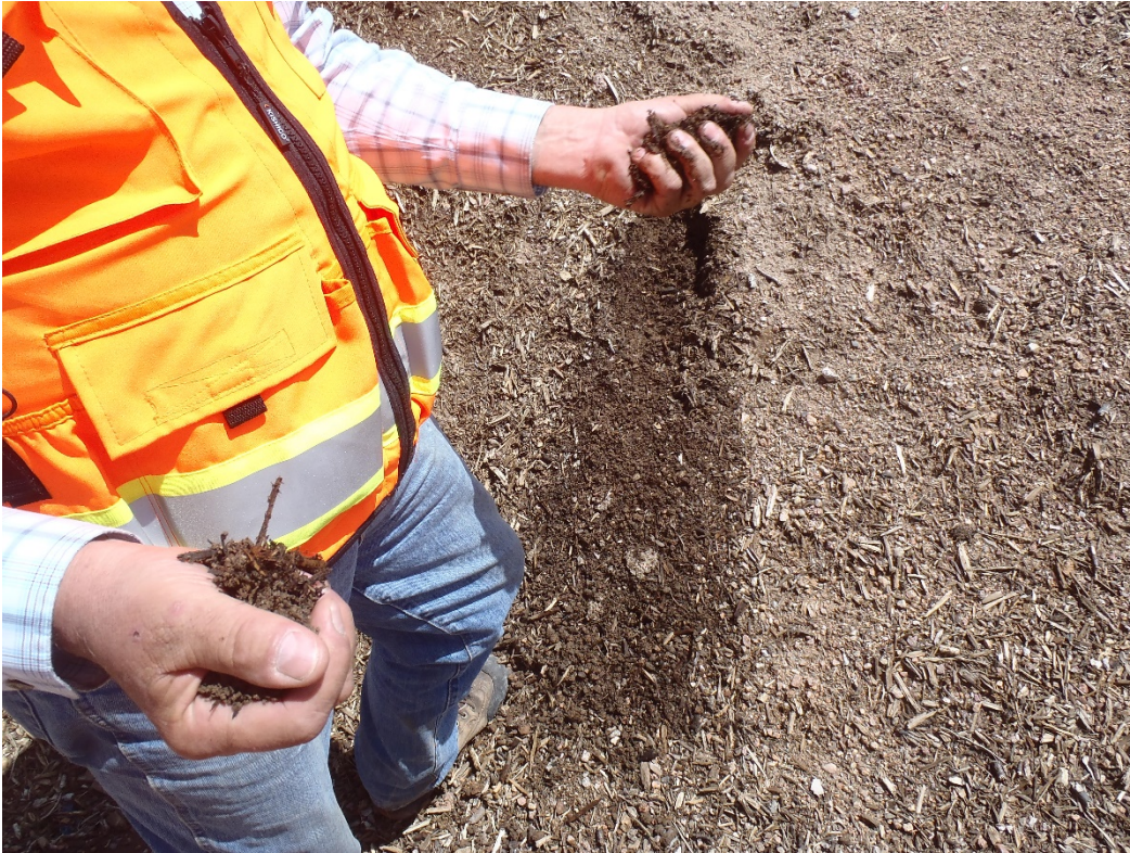
Photo 7. Mulch used to mix with on-site soils.
