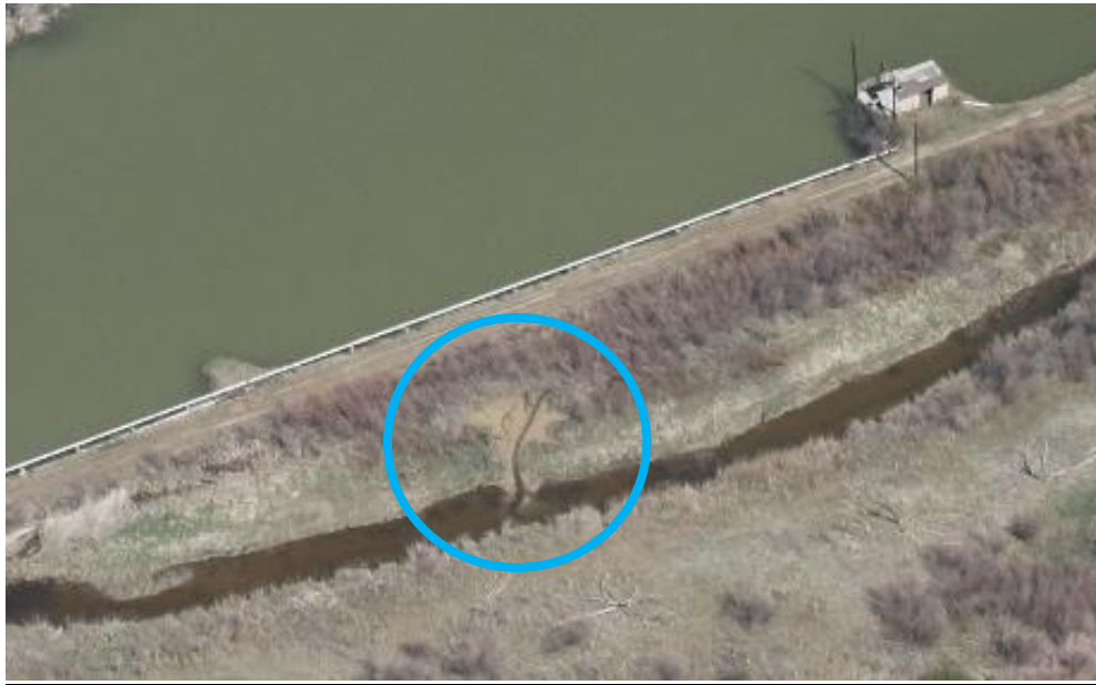
Photo 1a: A zoomed in view of the erosional feature next to the Raw Water Lagoon's south embankment.
