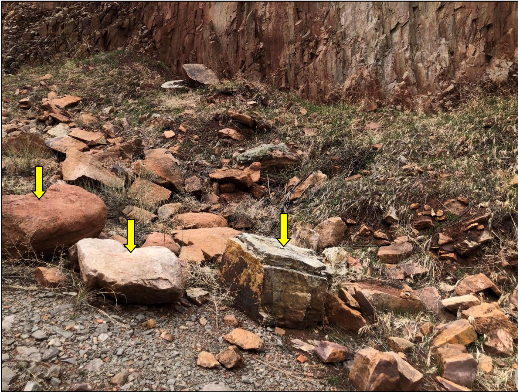
Photo 23. View looking southwest at Quarry 2, showing talus at foot of western highwall including rocks of various sizes, with larger boulders (up to 5 feet in length) typically derived from sandstone unit above dacite (a few of the larger sandstone boulders are indicated). Dacite rocks are typically smaller than 2 feet in length.
