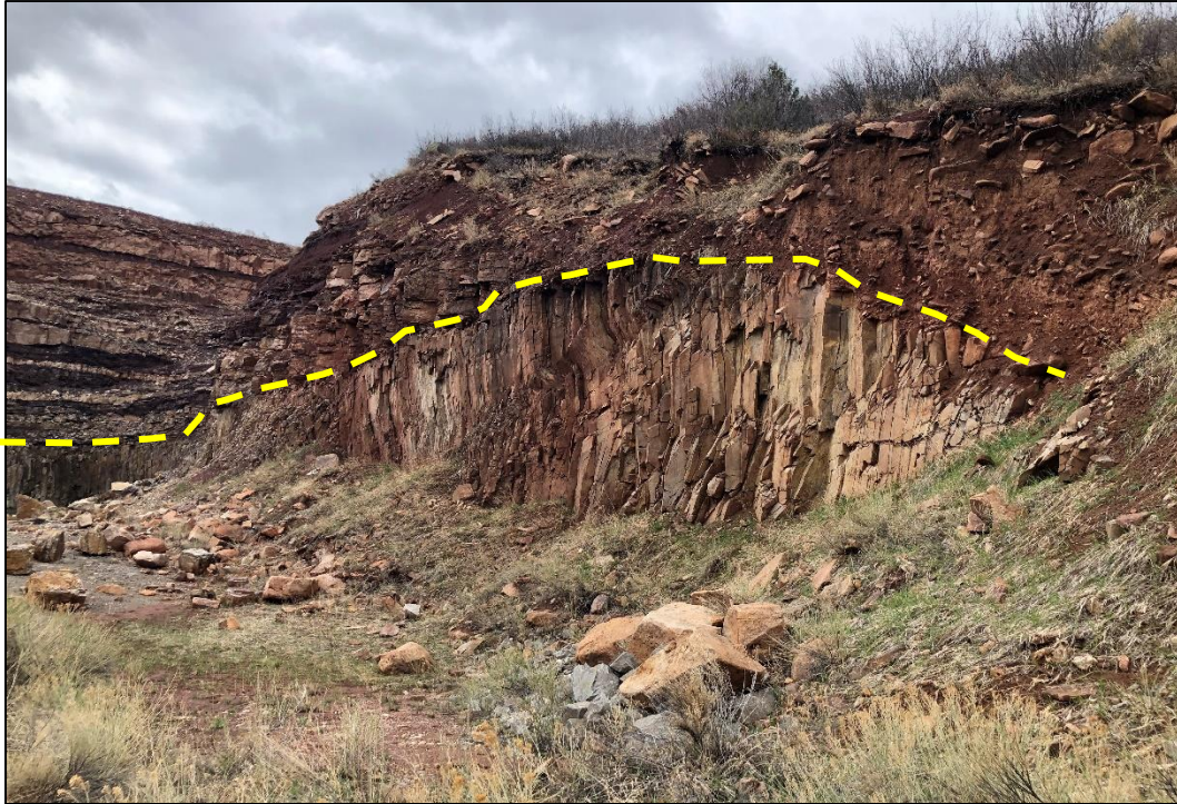
Photo 21. View looking southwest at Quarry 2, showing its western (northeast-facing) highwall. Note dacite rocks (lower portion of highwall) are heavily fractured. The approximate contact between the lower dacite and the upper sedimentary rock units is delineated with a yellow dashed line. Talus at foot of highwall includes rocks of various sizes, with larger boulders (up to 5 feet in length) typically derived from sandstone unit above dacite. Dacite rocks are typically smaller than 2 feet in length.
