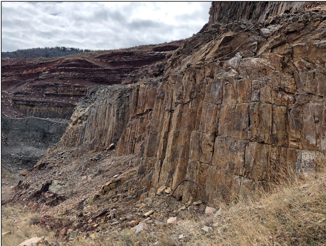
Photo 8. View looking southeast at Quarry 1 across lower (dacite) portion of its western (northeast-facing) highwall. Note dacite rocks are heavily fractured but dip mainly away from the quarry in this area, with slope gradients of near vertical to 0.5H:1V. Talus at foot of highwall includes rocks of various sizes, with larger boulders (up to 5 feet in length) typically derived from sandstone unit above dacite. Dacite rocks are typically smaller than 2 feet in length.
