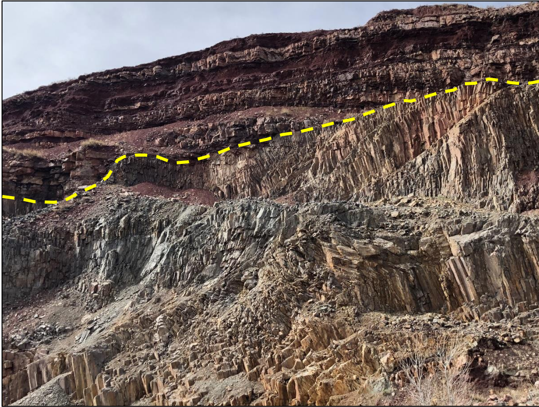
Photo 5. View looking southwest at Quarry 1, showing closer view of its western (northeast-facing) highwall. Note dacite rocks (lower half of highwall) are heavily fractured and dipping toward the quarry in some areas. The approximate contact between the lower dacite and the upper sedimentary rock units is delineated with a yellow dashed line.
