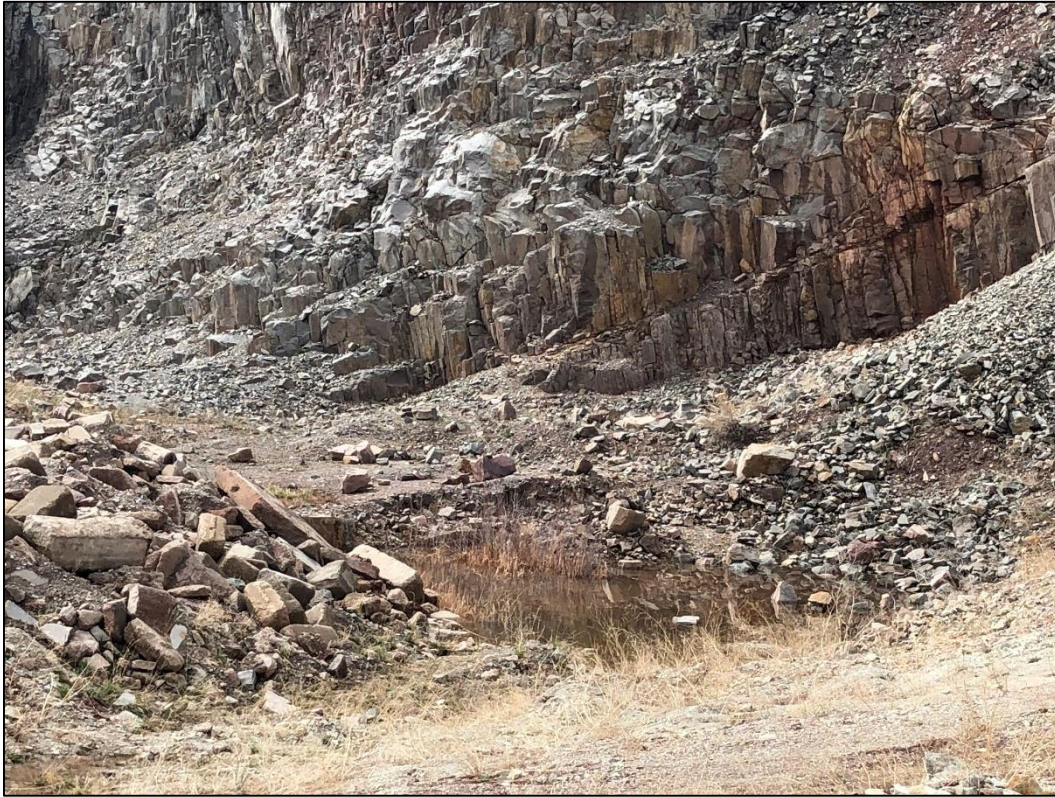
Photo 9. View looking southeast at Quarry 1 pit floor, showing talus present beneath highwall. Larger boulders (up to 5 feet in length) are typically derived from sandstone unit above dacite. Dacite rocks are typically smaller than 2 feet in length. Ponding shown in photo was from recent storm event.
