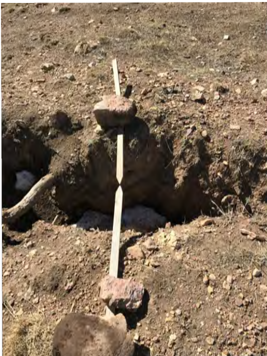
7. HISTORIC CRACK PARALLEL TO SLIDE
