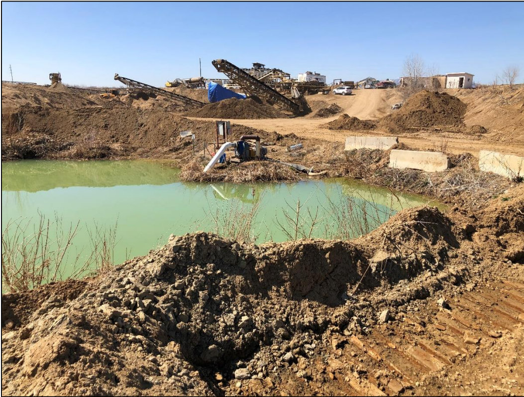
Photo 9. View looking west across western portion of Reservoir #4 pit, showing one of two settling ponds (in foreground), and processing plant (in background).
