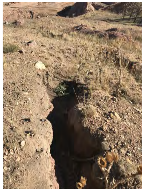
7. OPEN CRACK PARALLEL TO SLIDE
