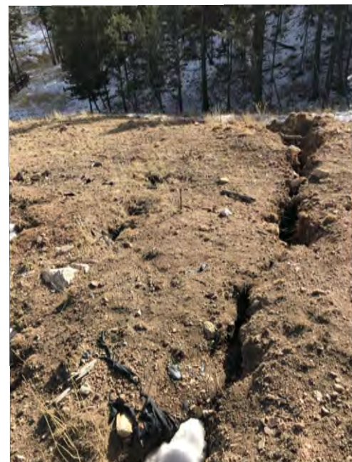
7. OPEN CRACK PARALLEL TO SLIDE
