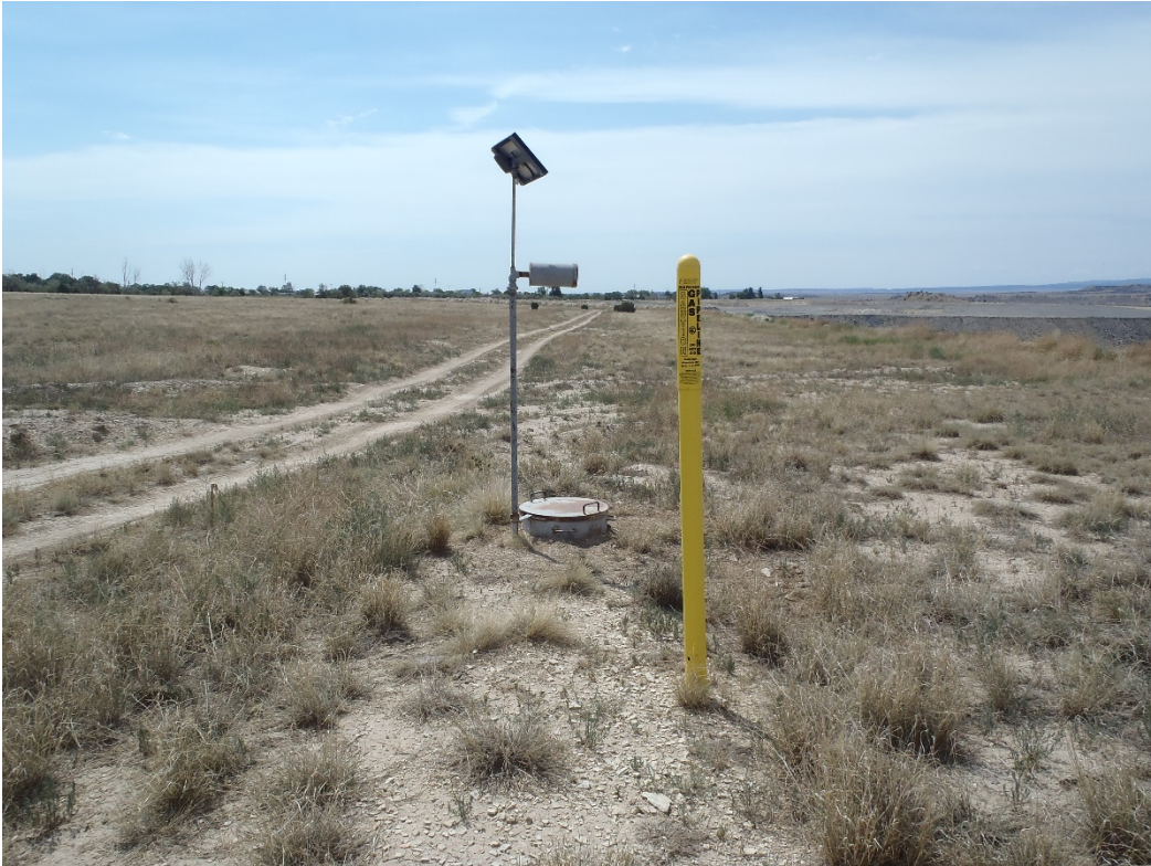
Photo 3. Permanent seismograph near gas line (north side, looking SE).
