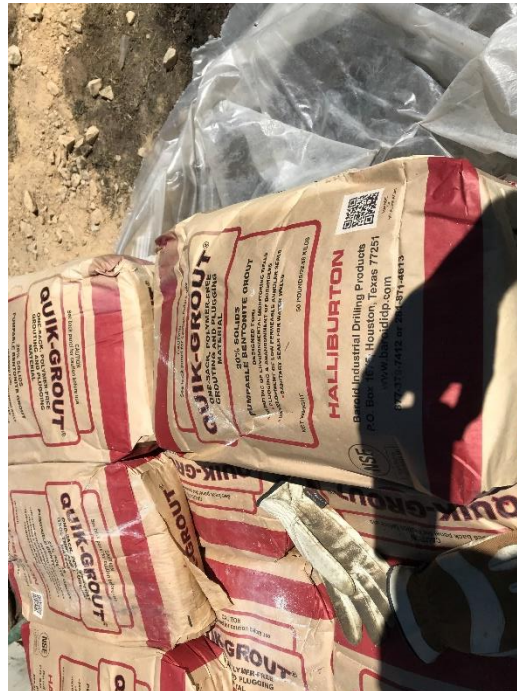
4. Grout plugging material used to abandon WP-6 Borehole
