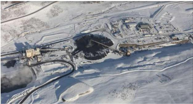
Shown below is the rest of the facilities area on the west side; pond B, pond C appear snow covered. BOB pile is on the left of the photo. The BOB pile topsoil pile appears stable and undisturbed. Truck and train loadouts are on the top right.
