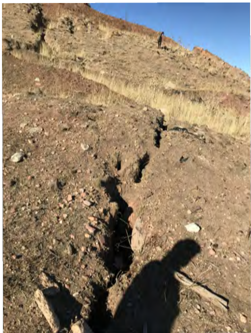
7. NEW CRACK PARALLEL TO SLIDE
