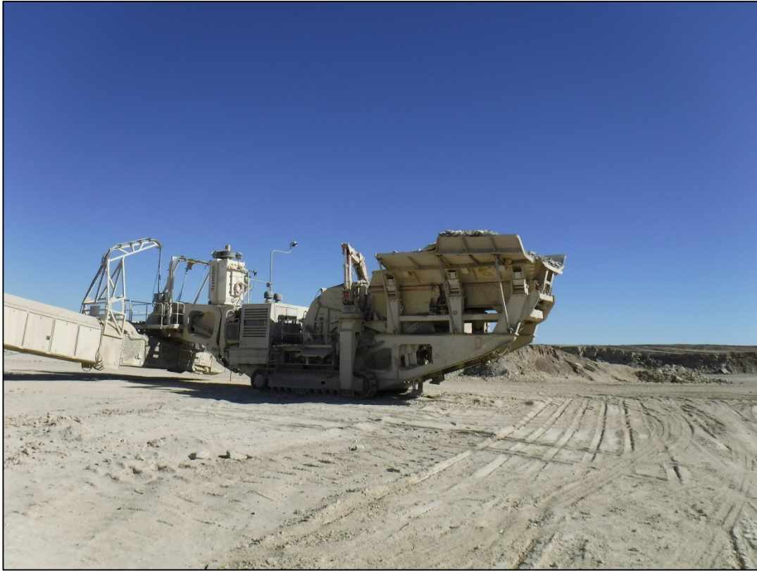
Photo 9: Mobile crusher/screener near active mine area
