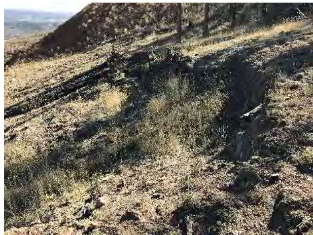
6. HEALED CRACKING ABOVE THE SLIDE AREA
