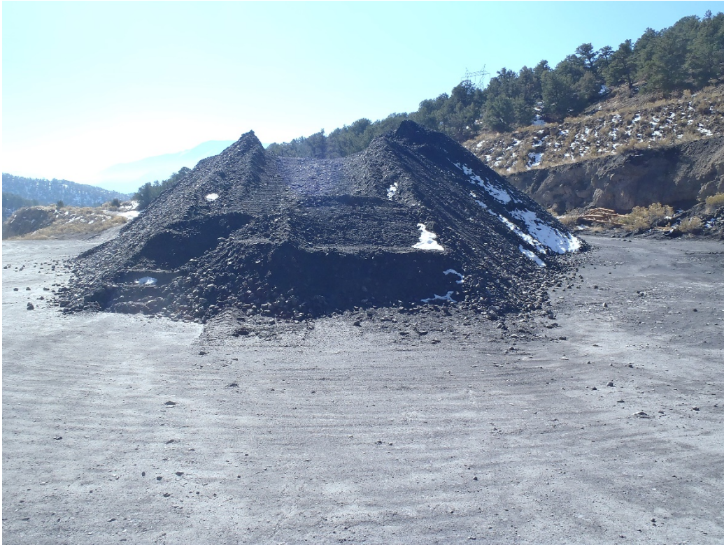
Photo 4. Blasted, crushed & screened material containing product awaiting haul to Wellsville plant.
