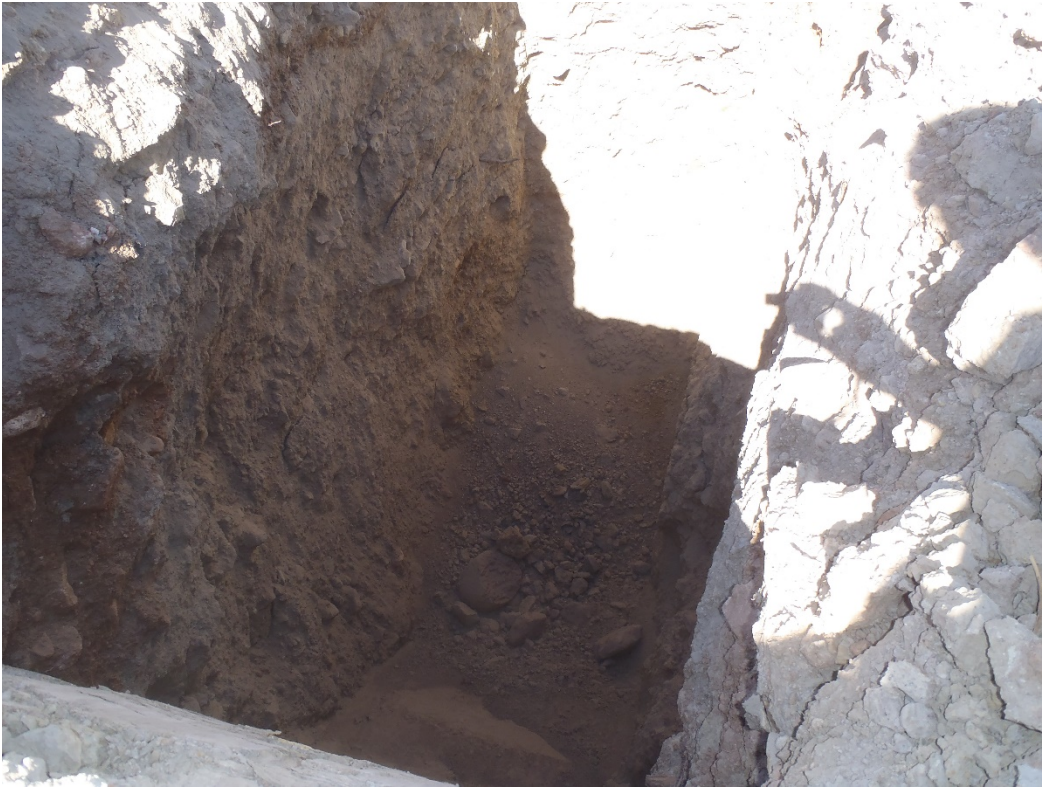
Photo 3. Test pit in "Area H" backfill (~12 feet deep).
