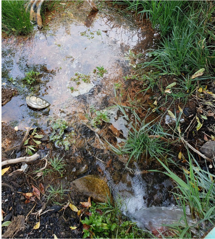
Figure 2 - Portal Discharge precipitate; only seen a few feet further than the pipe and not seen in any other ditch or pond.
