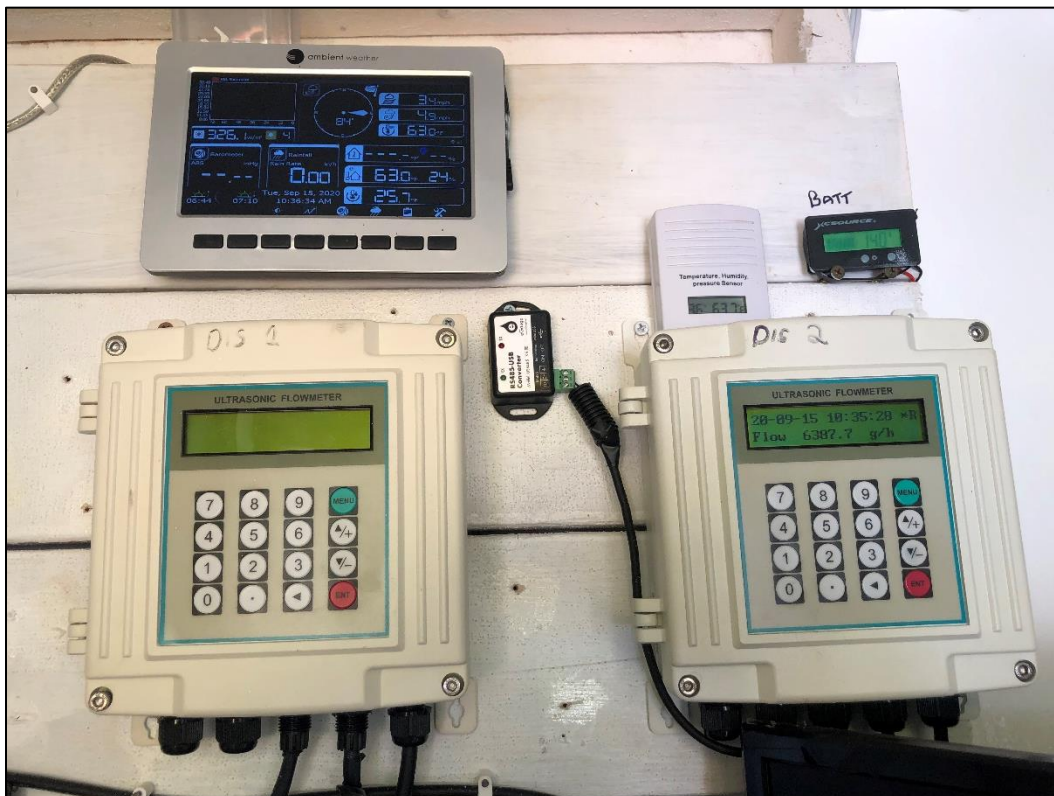
Photo 20. View inside new discharge shed through which discharge water from Pond 2 flows prior to discharging into Coon Track Creek under NPDES permit. Weather data and flowrate of discharge is measured at this station. Pond 2 discharge rate was 106.5 gal/min during inspection.
