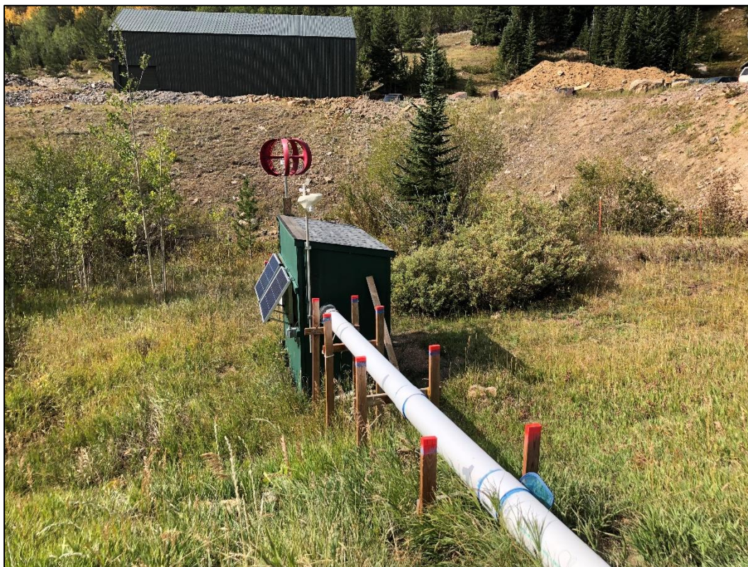
Photo 19. View looking south at new discharge shed located south of Pond 2 through which discharge from pond flows prior to discharging into Coon Track Creek under NPDES permit. Weather data and flowrate of discharge is measured at this station.
