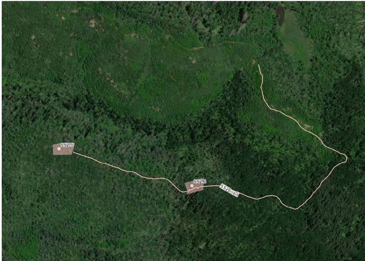
Figure 1: Features collected in the field using handheld GPS, showing locations of constructed road and pads, overlain on aerial image (credit: Esri)
