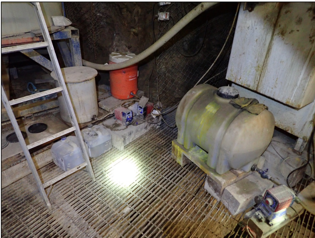
Photo 8. Mixed xanthate storage containers and pumps on upper level of mill.
