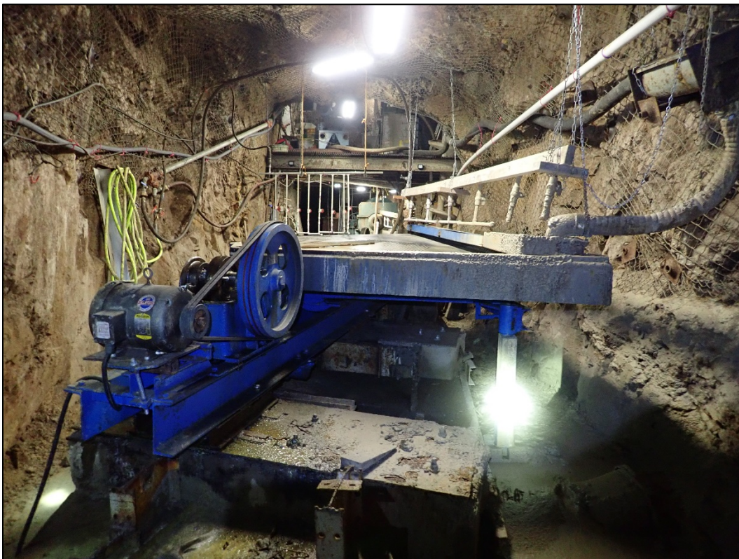
Photo 10. First of two gravity separation shaker tables on lower level of mill.
