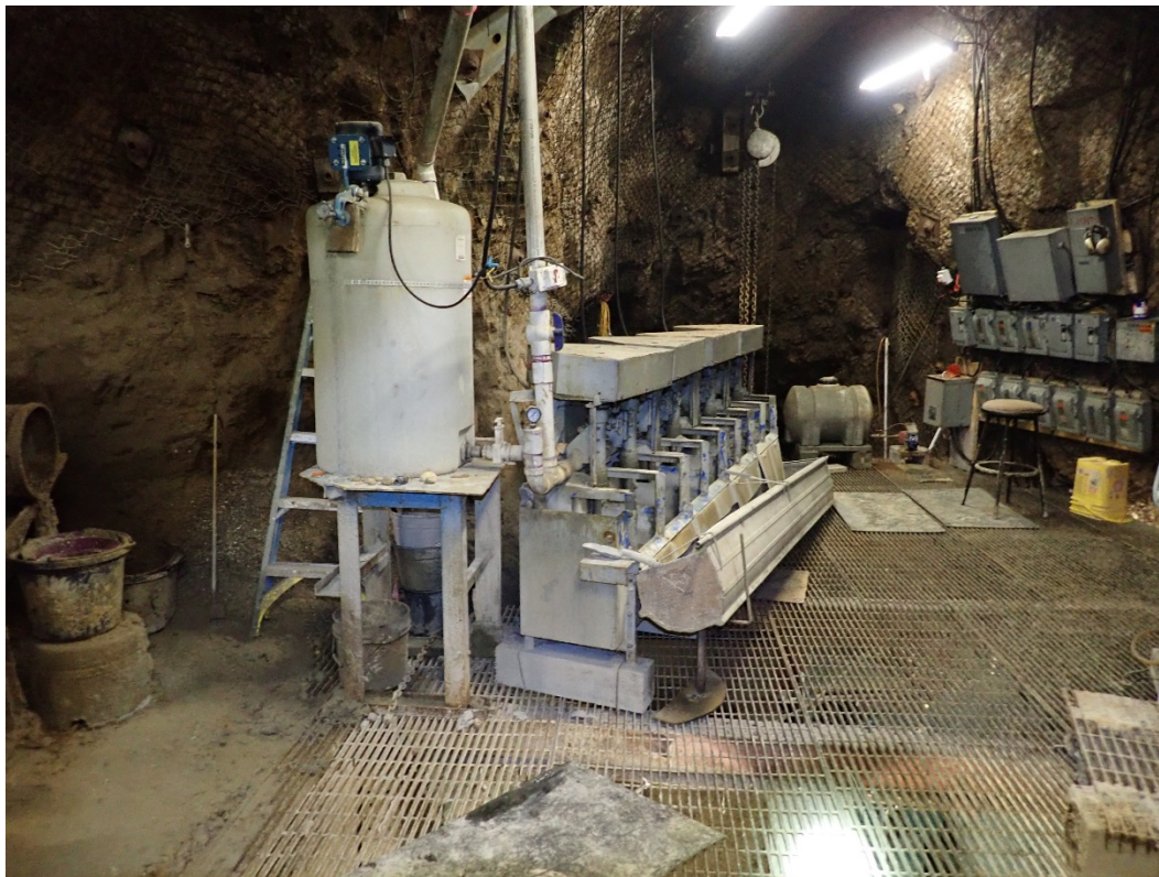
Photo 6. The second of two floatation machines on upper level of mill.
