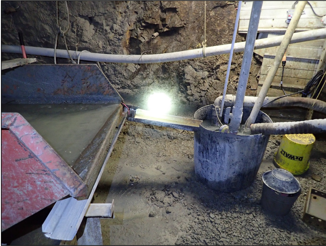
Photo 13. Regrind bucket collection and flotation concentrate settling bin on lower level of mill.
