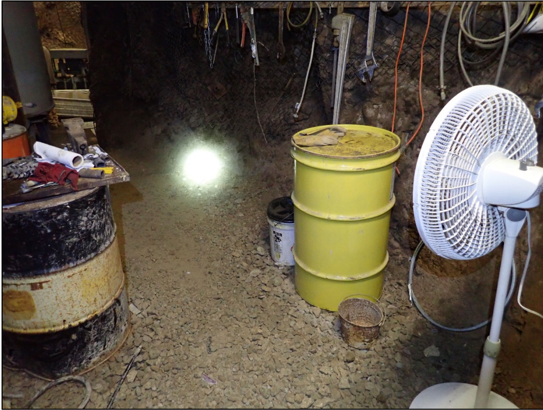
Photo 7. One of two 55 gallon drum of xanthate stored on upper level of mill.
