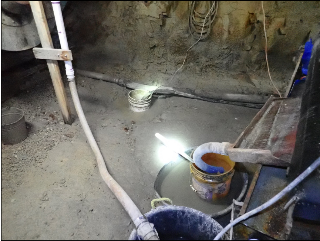
Photo 11. Gravity concentrate and gravity reject collection buckets after the second shaker table on lower level of mill.
