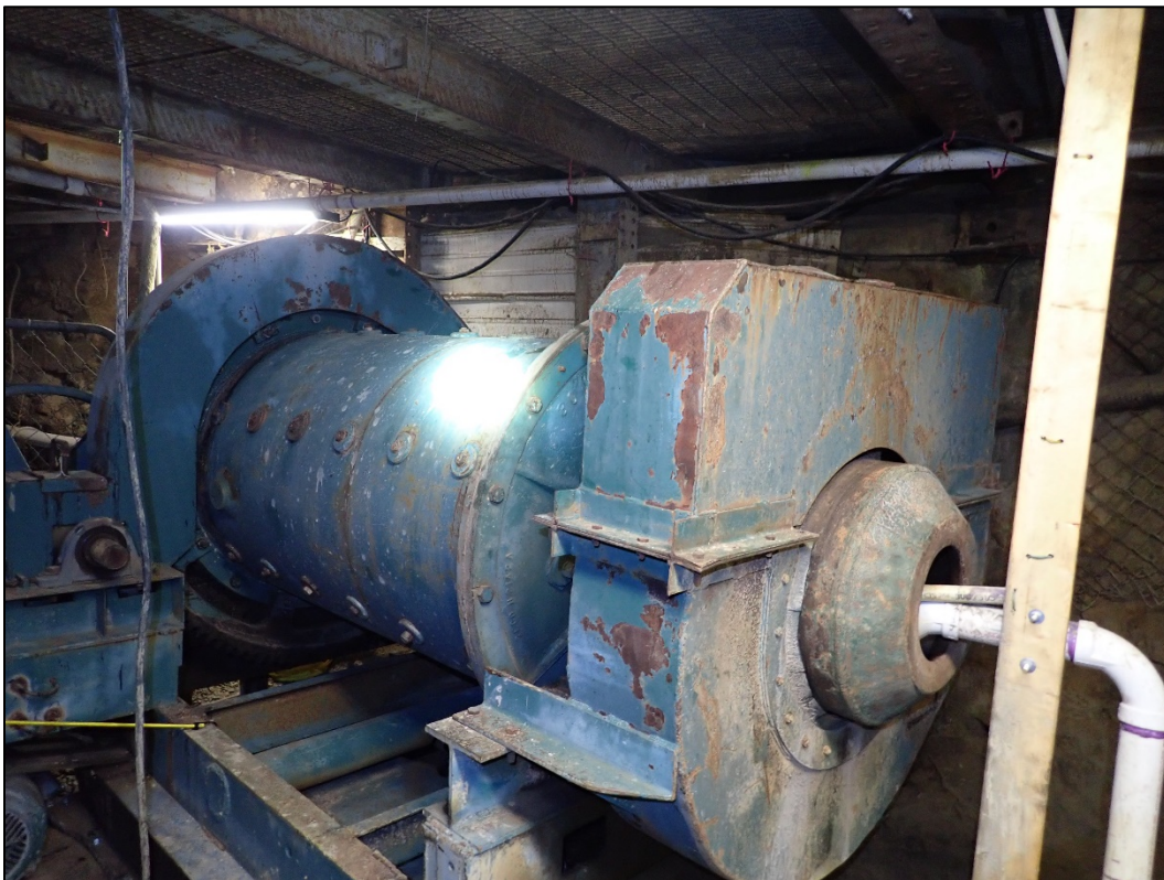
Photo 12. Regrind ball mill for gravity reject (start of the floatation circuit) on lower level of mill.
