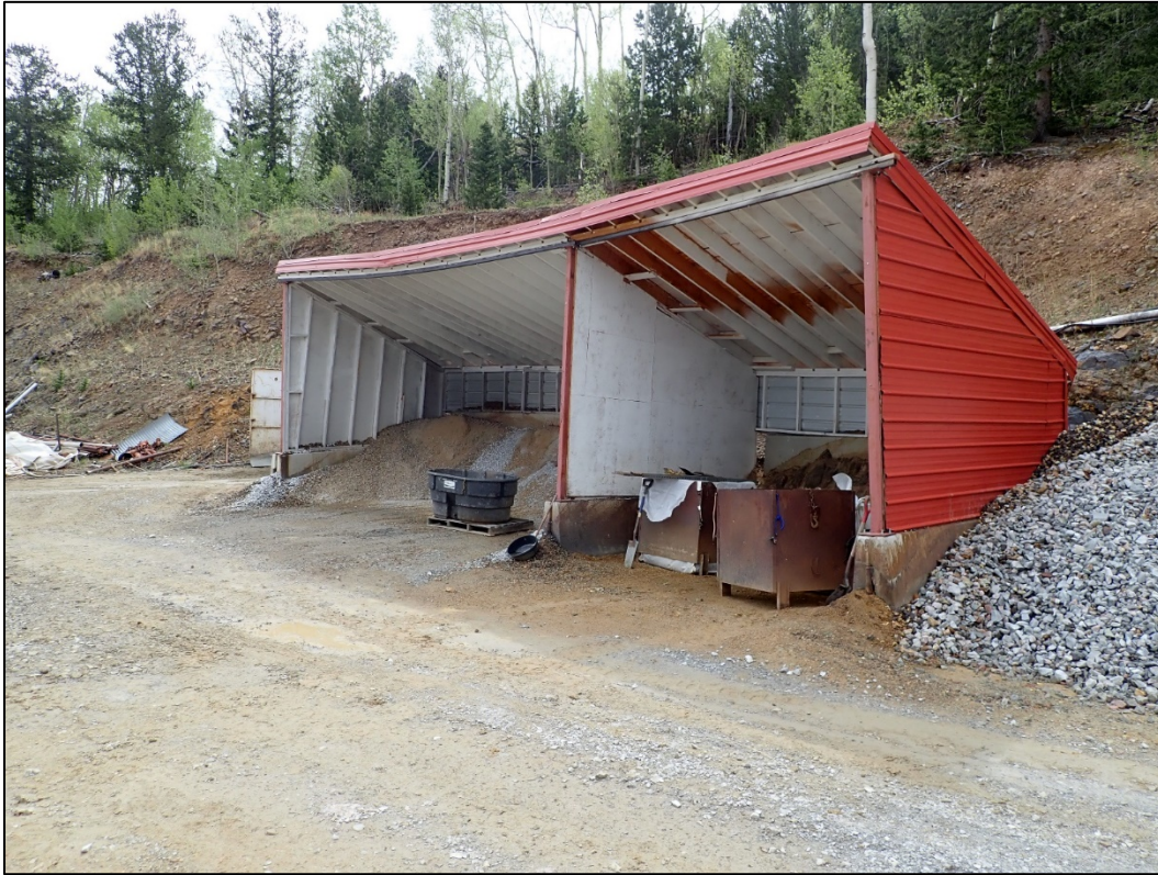
Photo 5. Open-sided building containing crushed ore (left) and gravity concentrate (right); looking southeast.
