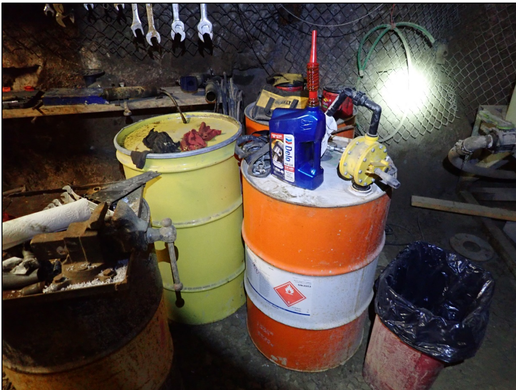
Photo 8. Second 55 gallon drum of xanthate and one of two 55 gallon drum of MIBC frother on upper level of mill.
