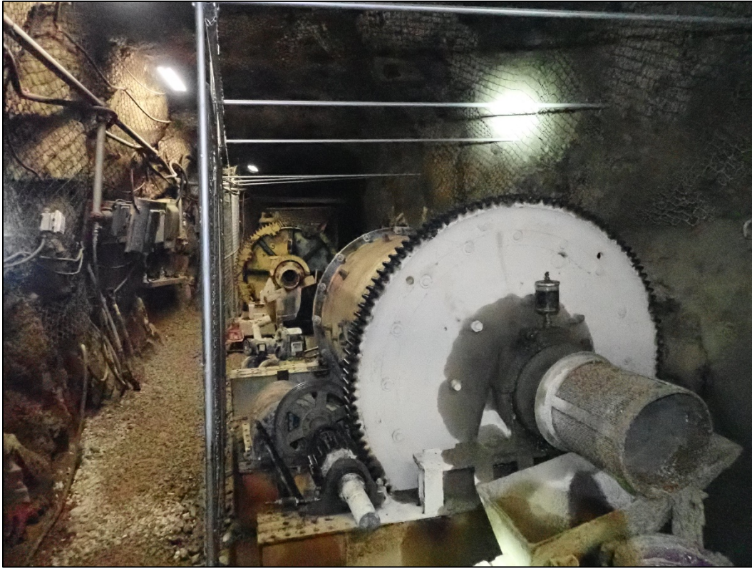
Photo 5. Two ball mills on upper level of mill.
