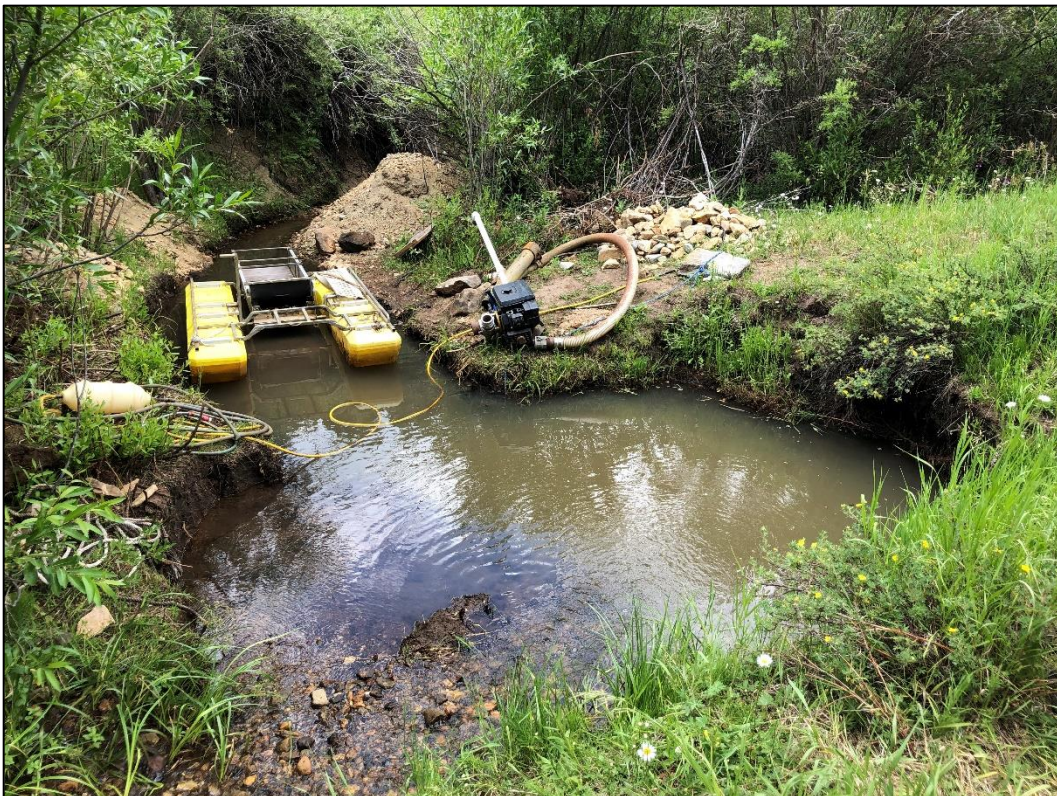
Photo 8. View of larger (8 foot wide x 8 foot deep) hole present in Beaver Creek in downstream section of creek disturbed by suction dredge operation. Note dredge equipment present on site and tailings piles stored along creek banks (in background).
