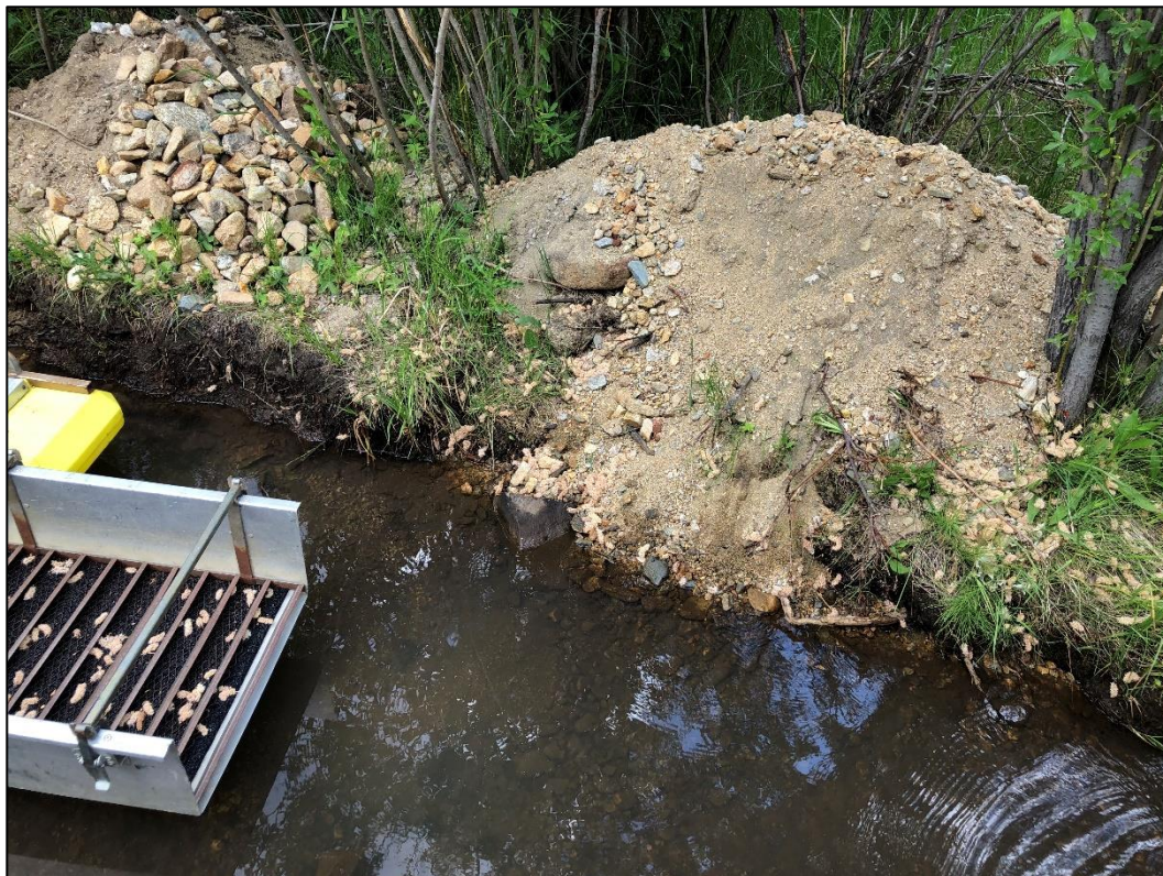
Photo 10. View of tailings piles left along creek bank by suction dredge operation.
