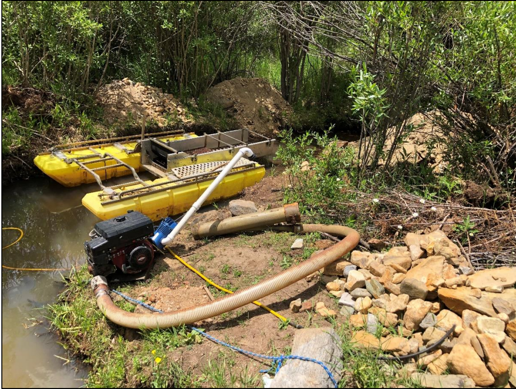
Photo 9. View of suction dredge equipment present on site. Note pile of larger rocks (at bottom right) pulled up from creek during dredge operations. Also note tailings piles stored along creek banks (behind dredge).
